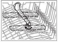
Wash the spray arm under running water. Use a thin pointed tool, e.g. a toothpick, to remove particles of soil from the holes.
