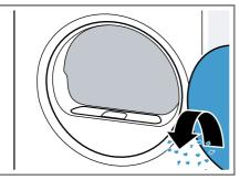
3. Remove the two-part fluff filter.
