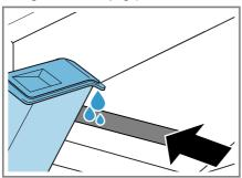
Check the water tank filter regularly and clean the filter if it is dirty. → "Cleaning the water tank filter", Page 38
